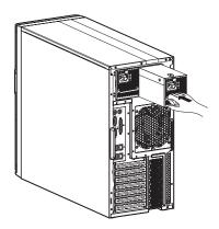
Werify that the power status indicators on the main power supply and on the newly installed redundant power supply are illuminated green.
